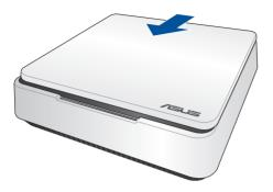
14. Lock the latch to securely fasten the top cover to the chassis.
